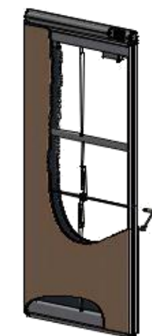
Manual locking system - 3S - locking of panels by one rotation of crank by 180°
